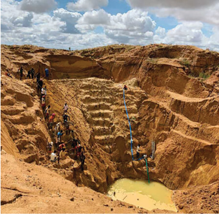
Each worker is forming a chain to get the earth out of the mine in Madagascar.
